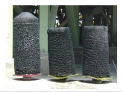
Pigs run through a 6" line. Left pig: type RBS. Right two pigs: type YBS. Polyurethane coating at base shows original diameter.
