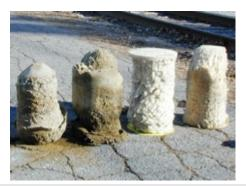
Pigs run through a scaled 8" water line. Left two pigs: medium hardness type RBS. Right two pigs: soft type YBS.
