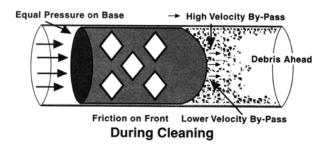
The cleaning action of the Girard Polly-Pig is created by the frictional drag provided by the oversize diameter. In addition, the pressure created by the fluid on the rear of the pig compresses the pig longitudinally. This increases the frictional drag on the walls of the pipe and the pig's scraping action.
