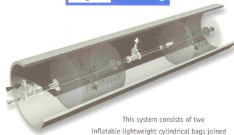
together by a semi-rigid or rigid spinal tube. The spinal tube carries an inflation supply to both bags and also acts as an argon gas feed to the space between the bags. The objective is to provide an inert atmosphere between the bags to enable a highquality weld to be carried out on stainless steel or other pipes where this type of atmosphere is recommended.
