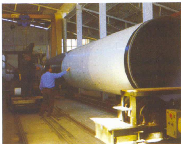
Water pipe (Acqueduct) diam 1600 mm. Altene Rp2 plant system
