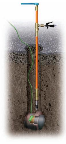
Long reach tooling enables operations to be conducted on underground gas pipes from surface level through a small 'keyhole' excavation. Keyhole excavation offers significant financial savings, reduced disruption to traffic and lower risk of damage to other buried plant.
